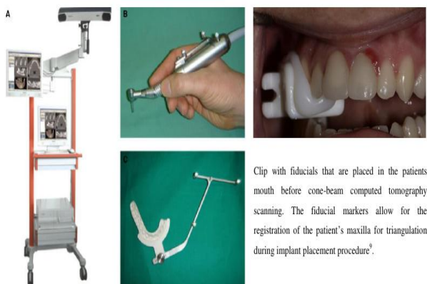
Fig 2: Components of Dynamic navigation (11)
